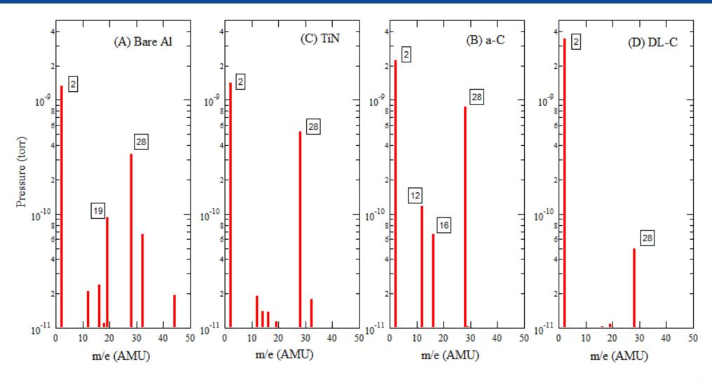
RGA Spectra of Well-Conditioned Chambers with ~400 mA Stored Beam @ 5 GeV
